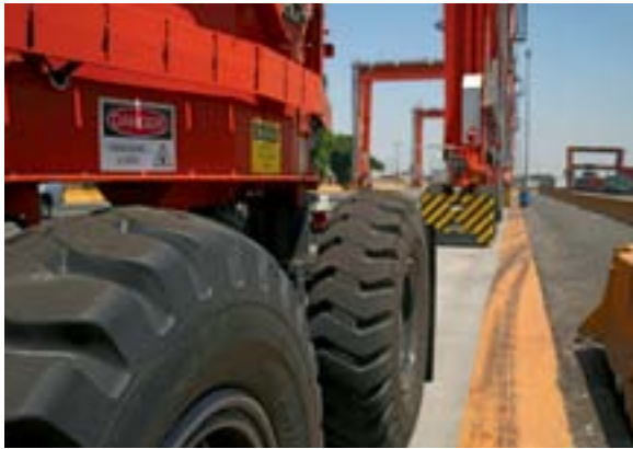
The new cranes at Los Angeles terminal are able to turn their tires ninety degrees, which improves their flexibility.
