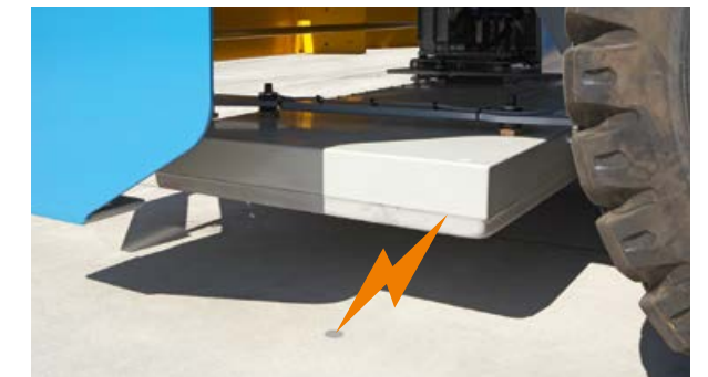
The transponder system, familiar from the Konecranes Gottwald AGV, is based on passive transponders in the terminal ground and surface antennas on the equipment side
