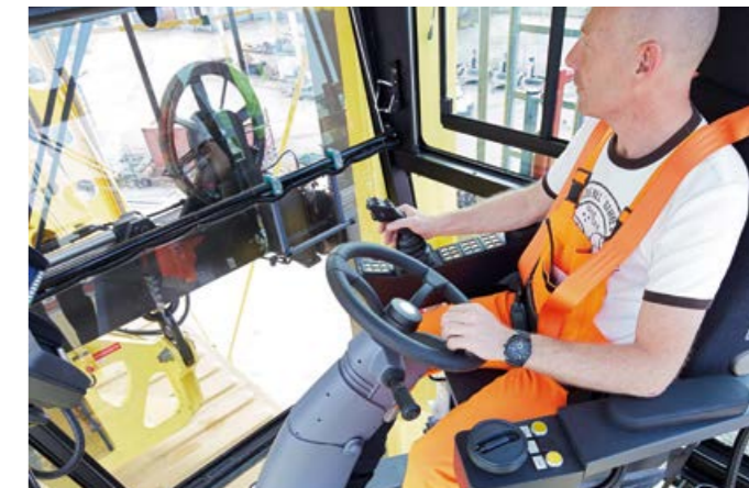
A cockpit that drivers like to work in: adjustable steering columns; electrically rotatable driver seat, on request; adjustable pedals.
